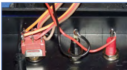
Fig.4.23 Rear panel wiring
