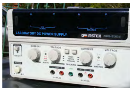
Fig.3. Dual-rail tracking bench power supply. Ideal for safe power-amp development. (GW-Instek GPS-2303 Rapid 90-6123).
