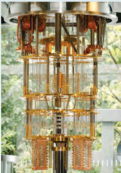
An IBM cryostat wired for a 50-qubit system.
