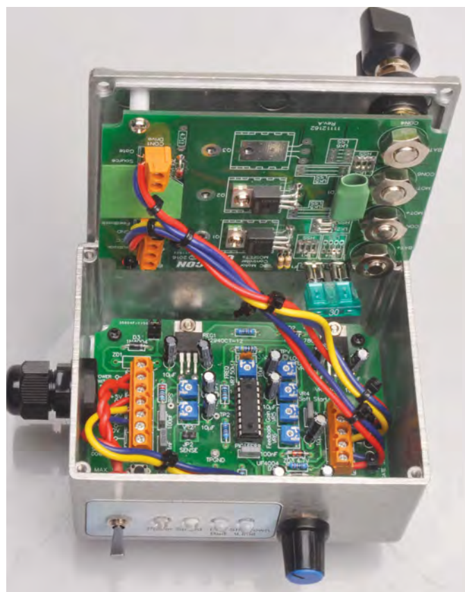
Inside the DC Motor Speed Controller – full construction details will be presented next month but will be slightly different from this prototype. The links on the motor PCB have been set up for high-side operation.
