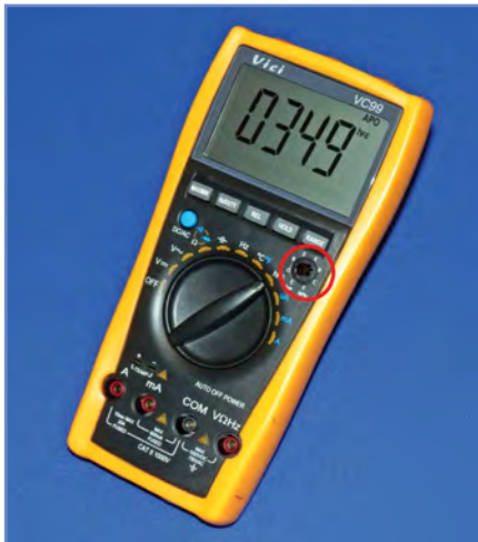
Fig.4.17 A low-cost multimeter being used to measure the current gain of a small-signal transistor inserted into the test socket (on the right-hand side of the instrument). The instrument is indicating a current gain ( h_{FE} ) of 381
