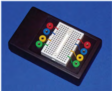
Fig.4.25 Breadboard test fixture
