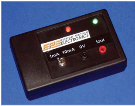
Fig.4.24 External appearance of the finished semiconductor junction tester
