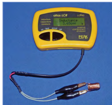
Fig.4.11 The Atlas LCR40 component tester being used to test a small toroidal inductor. The display is scrolled for additional information
