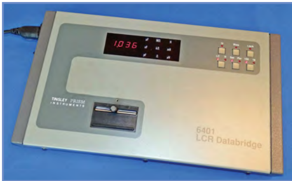
Fig.4.14 The Tinsley Prism LCR Databridge can measure a very wide range of resistance, capacitance and inductance with a basic accuracy of 2.5%
