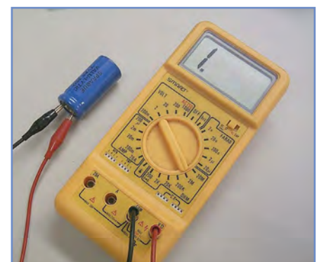
Fig.4.8 Measuring the insulation resistance of a capacitor with a multimeter is usually unsuccessful and invariably produces a meaningless over-range indication
