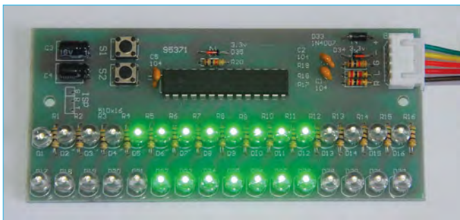
Fig.4. This display mode centres the displays, with the bar graphs extending further left and right to show greater levels.
