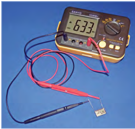
Fig.4.9 Using an insulation tester to check a Class X2 capacitor at an applied voltage of 1kV (well beyond the component's normal rating). After 60s of testing, the indicated value of IR is 633M \Omega
