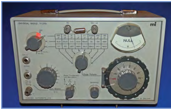
Fig.4.13 A Marconi Instruments TF2700 'universal' bridge being used to measure a polystyrene film capacitor. Note the 'null' meter, range switch and large adjustable variable control
