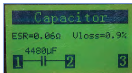
Fig. 4.5 Using a low-cost component tester to check capacitance (4480µF), ESR (0.06Ω), and voltage loss (0.9%)
